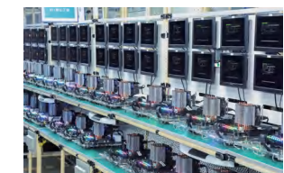
Functional Testing (BIWINSight proprietary testing software)
