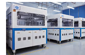
Fully Automated IC Screening Test (Environmental temperature range from 25 °C to 85 °C)
